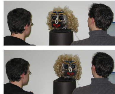
Figure 1: A conversation of our robot Alpha with two people. As can be seen, the robot shifts its attention from one person to the other to involve both into the conversation.
