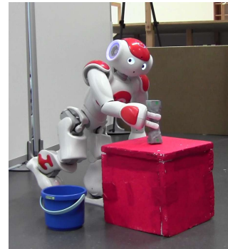
Fig. 1. Imitation of a complex whole-body motion with a humanoid for a tele-operated manipulation task. Note that the robot imitates configurations in which it is required to balance on one foot over a longer period of time.
